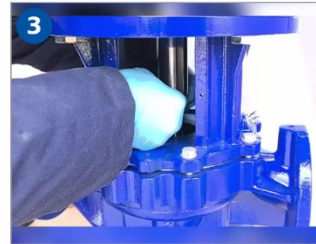
Withdraw the seal off the shaft
