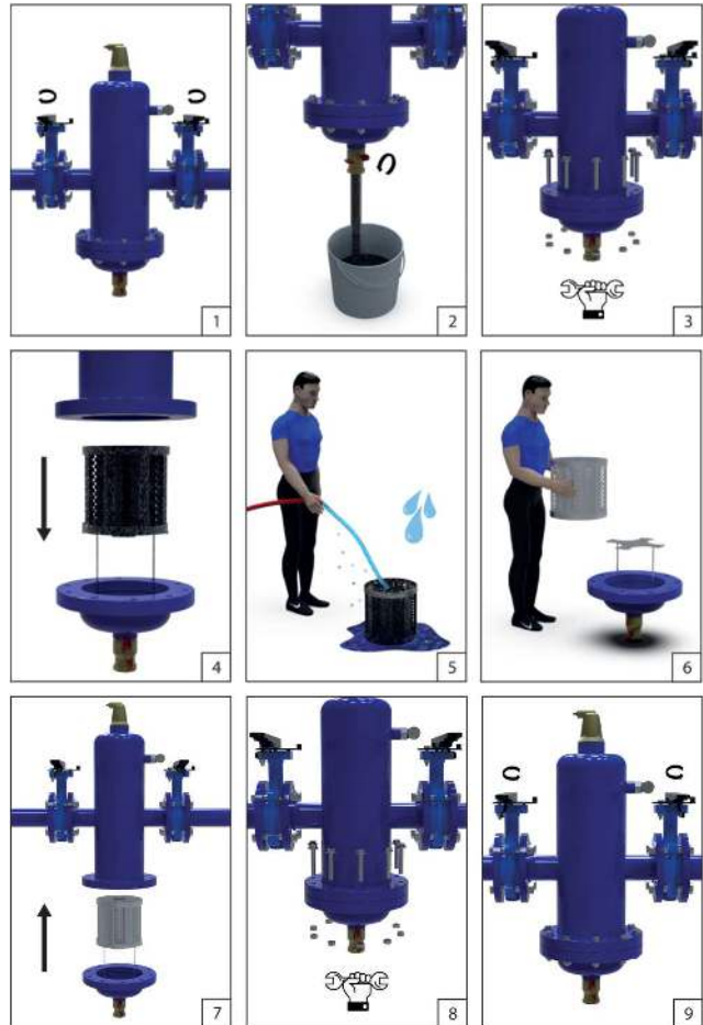
Fig: Demountable coalescing-element cleaning sequence
